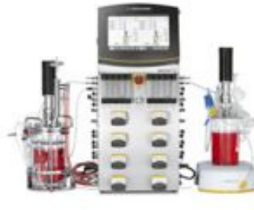
(a) StemSpan™ Spinner Flask (STEMCELL Technologies Inc). (b) BIOSTAT® B twin version with stirred glass vessel and with single-use vessel (Sartorius).
