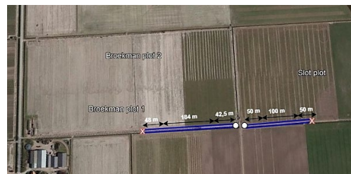
Figure 5 - Top-view of the agricultural plots identifying the location and length of the injection wells
