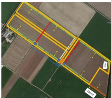
Figure 3 - Top-view of the drainage systems, with the drainage pumps in blue, the drainage pipes direction in yellow and the collector drains in green
