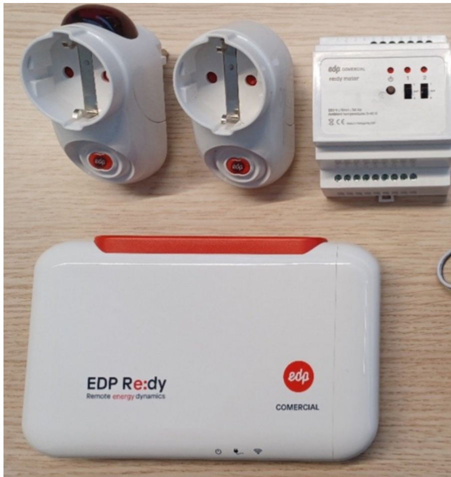
Figure 2.1: An ensemble of edp re:dy products that can be used for the home monitoring purposes. source: https://www.sato-project.eu/news/edp-new-completes-demonstration-activities-in-seixal-residential-pilot
