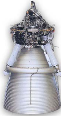
Fig. 0.1 – Vulcain 2 rocket engine, from Astrium, that powers the Ariane 5 (LOX/LH 2 ). With regenerative cooling system that supports the combustion chamber and also the active cooled nozzle by dump flow.
