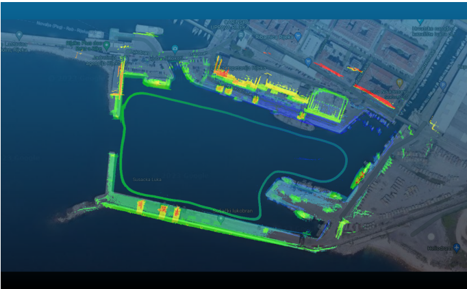
Fig. 5. 3D SLAM generated map overlaid with Google Maps screenshot - Rijeka Harbour dataset
