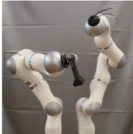
Figure 3.25: Two KUKA LWR IV robotic arms extant at the Control, Automation and Robotics Laboratory of Instituto Superior Técnico, Universidade de Lisboa, Portugal. Each robot has seven rotational joints. (Source: Professor Jorge Martins.)
