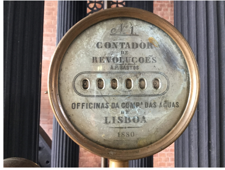
Figure 3.12: Mechanical 19th century revolution counter, from the former Barbadinhos water pumping station (currently the Water Museum), Lisbon. Nowadays mechanical revolution counters are still used, though electronic ones exist.
