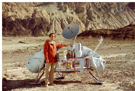
Figure 3.24: Astronomer Carl Sagan (1934 – †1996) with a model of one of the two Viking landers, space probes that descended on Mars in 1976 and worked until 1980 and 1982 (source: Wikimedia). Descent speed was controlled by deploying a parachute and launching three retrorockets (one on each leg) to ensure a soft landing. The descent control system employed an inertial reference unit, four gyroscopes, a radar altimeter, and a landing radar.
