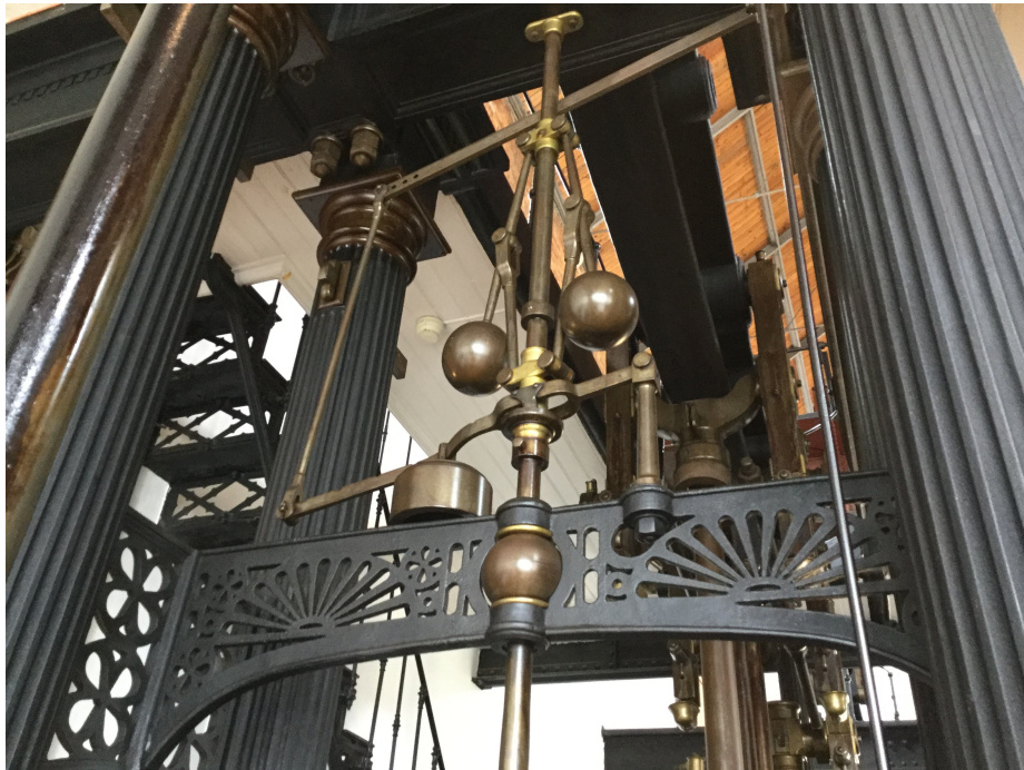
Figure 9.6: Centrifugal governor of a boiler in the former Barbadinhos water pumping station (currently the Water Museum), Lisbon.
