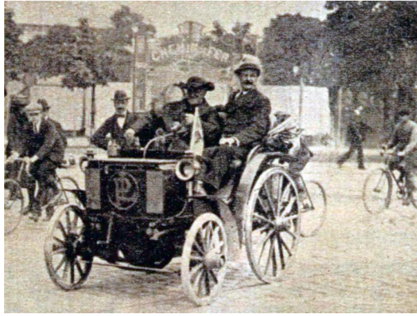
Figure 3.4: A Panhard & Levassor Type A motorcar, the first mass produced car in the world, driven by the French priest Jules Gavois (1863 – †1946) in 1891 (source: Wikimedia). This car still does not have a steering wheel (first introduced in 1894), but only a tiller.
