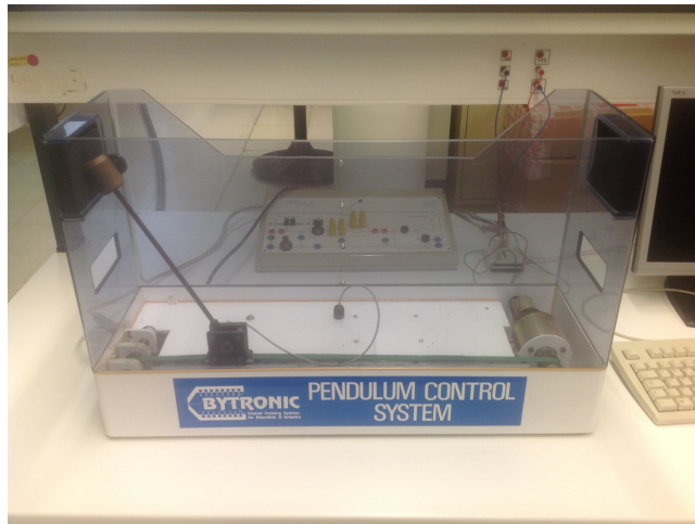
Figure 27.4: Inverted pendulum in the Laboratory of Control and Robotics; its parameters are not those of transfer function (27.4).
