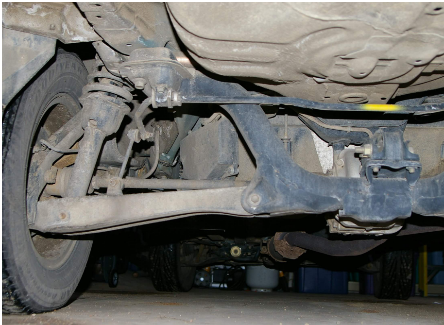
Figure 4.6: Independent suspension of a car's wheel (source: Wikimedia). The spring is clearly visible. The damper can be seen inside the coils of the spring. Even when the suspension does not consist of one spring and one damper, a mass–spring–damper model can be used, as nearly all suspensions have a spring-like restitution force and some sort of energy dissipation.
