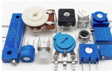
Figure 5.2: Potentiometers (or variable resistors, or rheostats) have a slider or a screw to move the position of a terminal, and thus the length of the resistor which is actually employed; resistance is proportional to this length (source: Wikimedia). See Figure 5.3.
