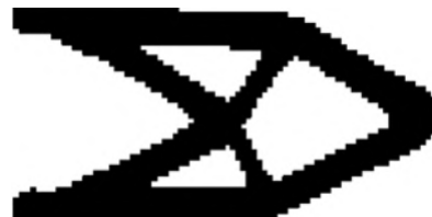
Figure 4.7: Optimum solution for the cantilever subjected to a point load [Kaveh et al., 2008].
