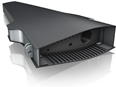
Figure 7.7: Conventional wing box.
