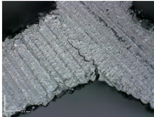
Figure 4.26: Crack initiation and propagation in a triple junction (sample L10H10).
