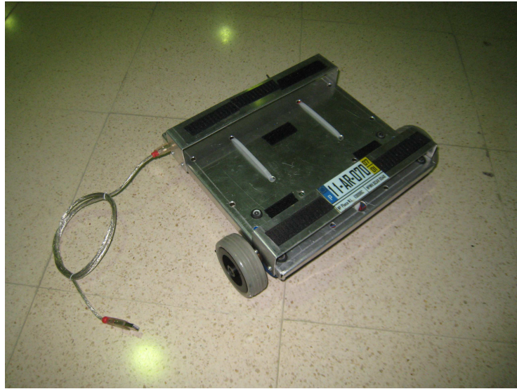
Figure 10.4: The Rasteirinho mobile robot, without the laptop computer with which it is controlled.
