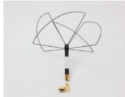
(b) Video Tx Skew planar wheel antenna [76].
