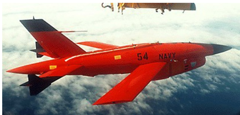
Figure 1.1: Jet-powered surveillance UAV Ryan Firebee [3].
