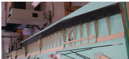
(a) Wing structure manufacturing.
