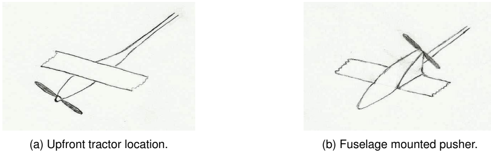
Figure 2.7: Sketches of possible engine sets.
