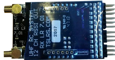
Figure 3.5: Long range radio receiver Thomas Scherrer Rx700. [71].
