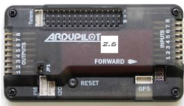
Figure 3.4: Autopilot Ardupilot APM 2.6 [70].
