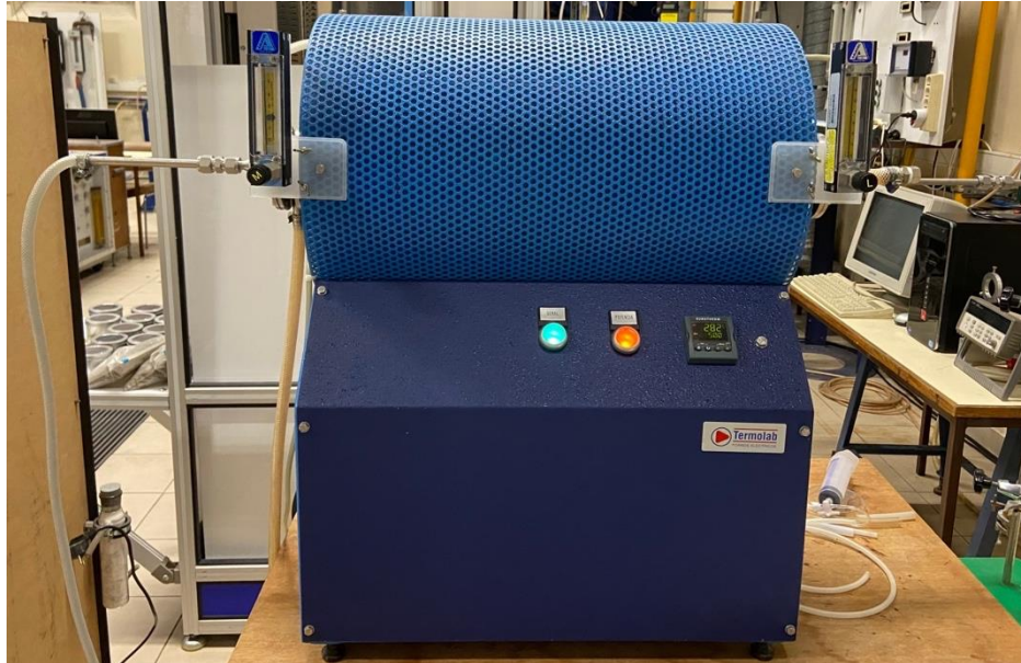
Figure 16. Horizontal tube furnace used for the slow pyrolysis process.
