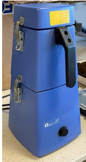
Figure 1. IKA-WERKE M20 mill used to grind the biowaste samples.
