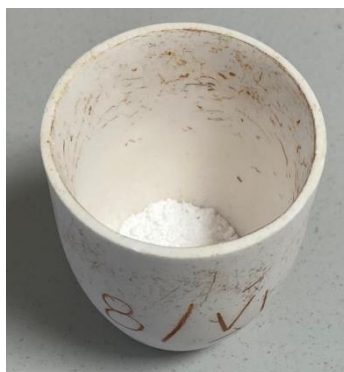
Figure 10. Sample prepared for determination of chlorine content.
