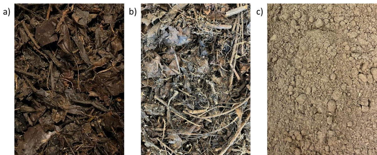
Figure 4. Autumn garden biowaste: a) before drying, b) after drying, c) after grinding.
