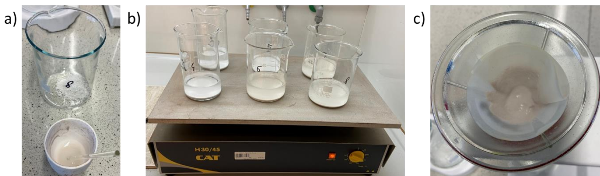
Figure 11. Sample preparation: a) transfer the content of the crucible to the beaker, b) boiling the content of the beaker, c) filtration.
