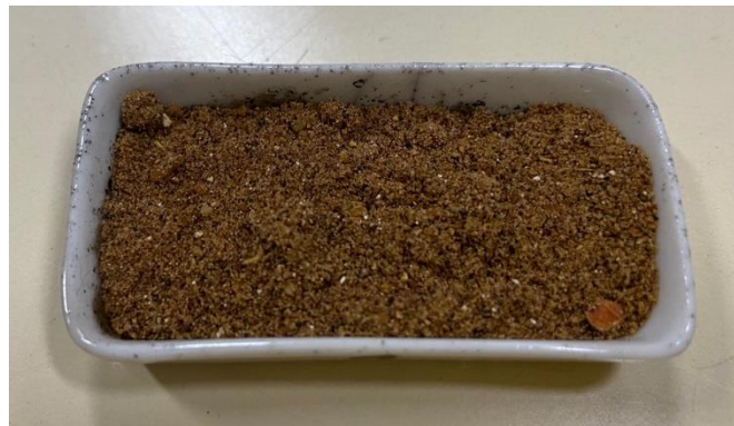
Figure 18. One of two crucibles containing a 2.5 g sample of kitchen biowaste prepared for slow pyrolysis.
