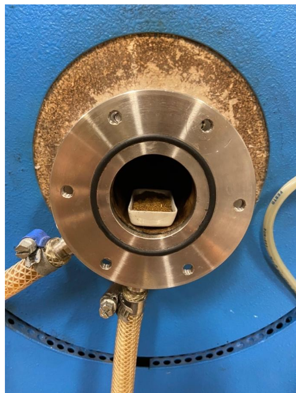
Figure 19. Crucible with sample placed in the horizontal furnace tube (after such placing, the crucible was moved to the center of the HTF).
