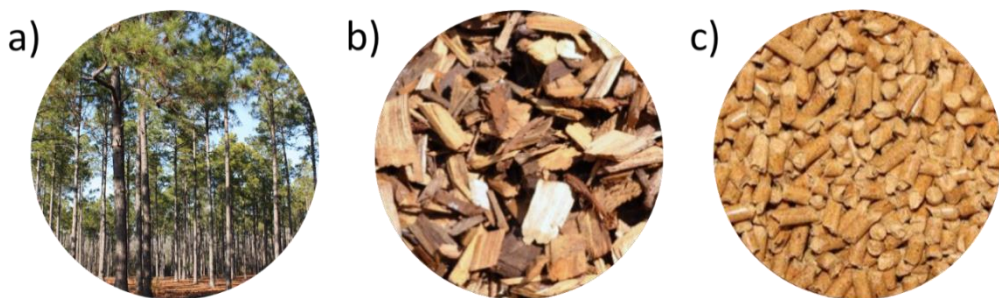
Figure 9. Biomass Feedstock at different stage: a) Pine trees; b) Pine woodchips; c) Pine pellets.
