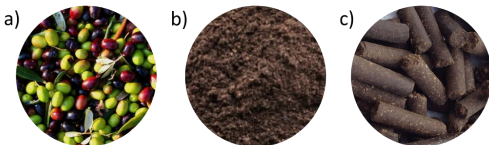
Figure 7. Biomass Feedstock at different stage: a) Olive's cultivation; b) Dried olive pomace; c) Olive pomace pellets.
