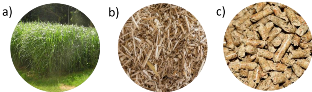
Figure 8. Biomass Feedstock at different stage: a) Miscanthus cultivation; b) Miscanthus harvested; c) Miscanthus pellets.
