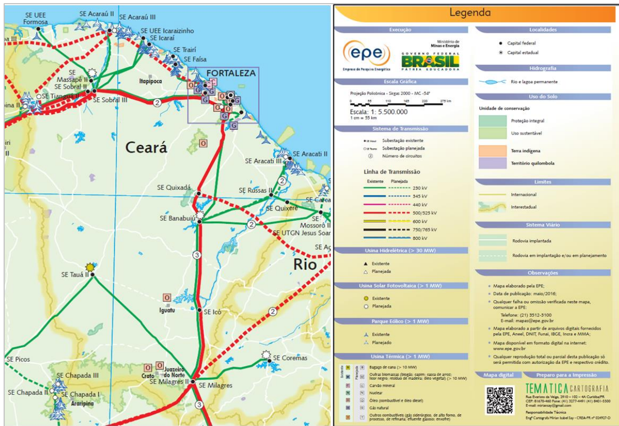
Figure 32: Ceará electricity transmission network, mapping of current and planned power plants and land use differentiation. Source: [76]
