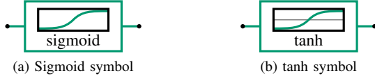
Fig. 9: Activation functions symbols with the input and output pins on either side depending on the flow of the current for better readability
