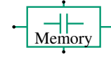
Fig. 12: Memory cell symbol with the input enable pin (top) and the output enable pin (bottom). The left and right pins are interchangeably the input and output for the sake of readability
