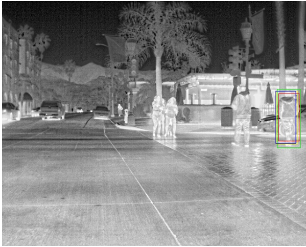
Fig. 7. Fused box (yellow): squared error = 10.817, NLL_{reg} = 693.187 . RGB box (blue): squared error = 14.353, NLL_{reg} = 523.103 . Thermal box (red): squared error = 17.176, NLL_{reg} = 208.560 . Ground-truth (green) for comparison.
