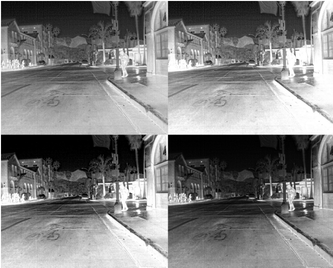
Fig. 5. Gamma augmentation (bottom-right) preserves more details than brightness (top-right) and contrast (bottom-left), even for large parameter values. Effects are noticeable on pedestrians on the left and right regions of the images. Top-left shows the original image for comparison.
