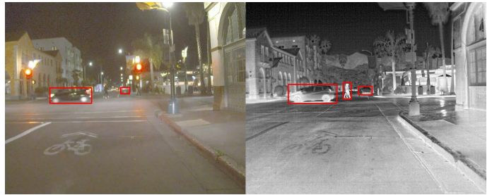
Fig. 1. Example of RGB/thermal image pair at night. A pedestrian was detected in the thermal image, but not in the RGB image.
