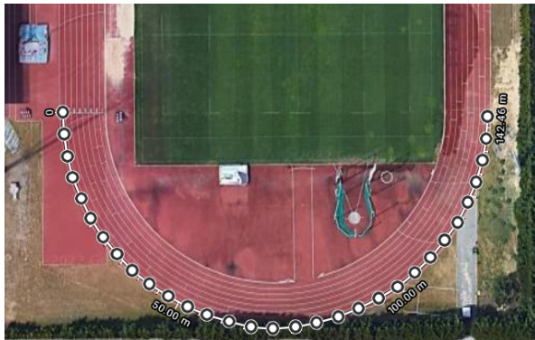
Figure 9: The track's semi-circle divided into 30 evenly spaced points
