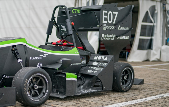
Figure 2.23: Example of FS car with side wing and side cascade
