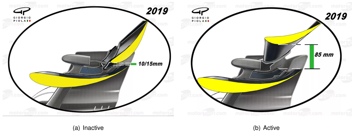
Figure 2.18: Drag Reduction System [39]
