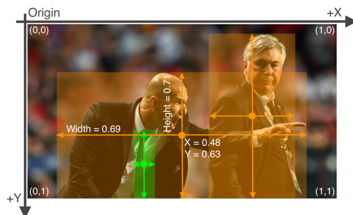
Figure 1.1: Sample image from Coco Dataset, representing the YOLOv5 Bounding Box Coordinate System [1]
