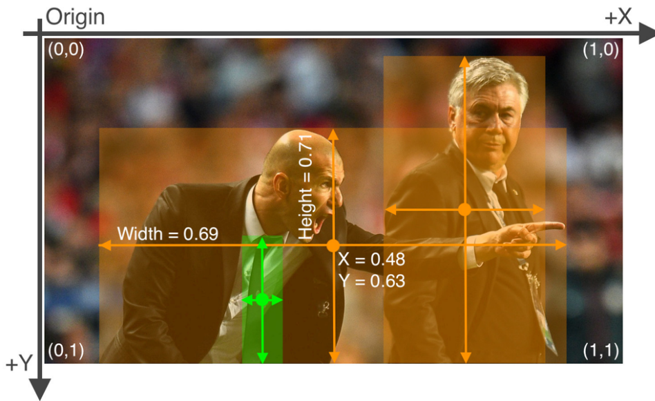
Figure 4.1: Sample image from Coco Dataset, representing the YOLOv5 Bounding Box Coordinate System [1]
