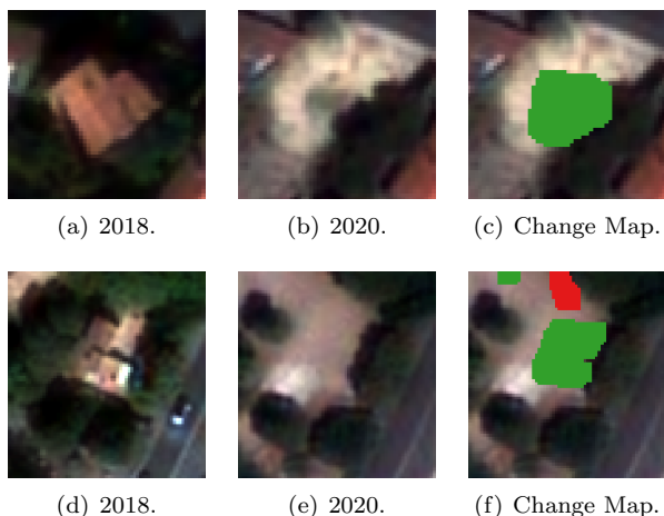
Figure 4: Close-up on images (in RGB) and artificialisation maps (green and red in change maps correspond to naturalised and artificialised pixels) of parcels 34172000KM0031 (top) and 34172000EZ0159 (bottom).
