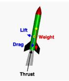
Figure 2.2: Forces acting on a rocket [17].
