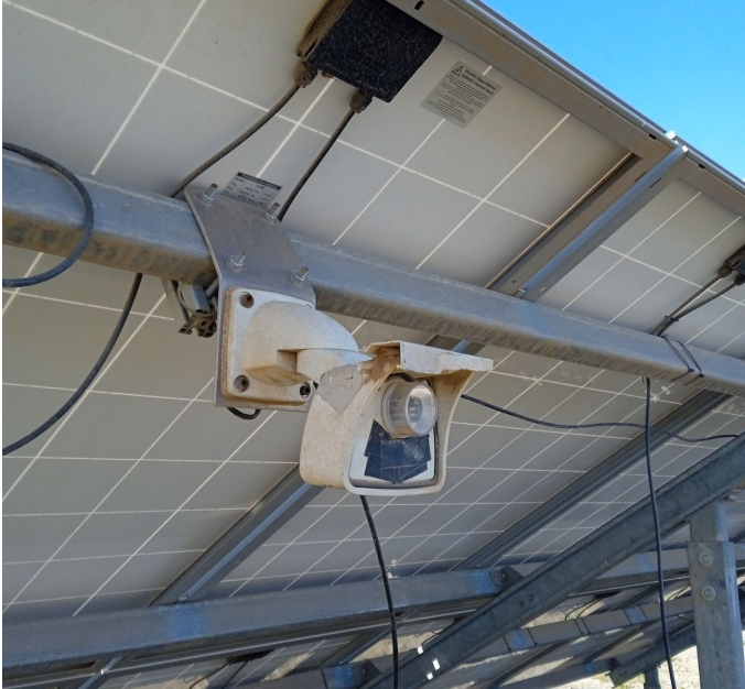
Figure 4.4: Surveillance camera. Mobotix MXM24M-Sec-D22, CMOS sensor [40].
