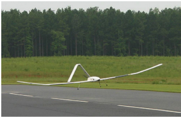
(a) FC-powered UAV, developed by Bradle et al. [68];
