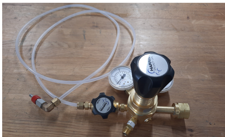
Figure 3.2: Harris KH1130 pressure regulator, with attached hose.
