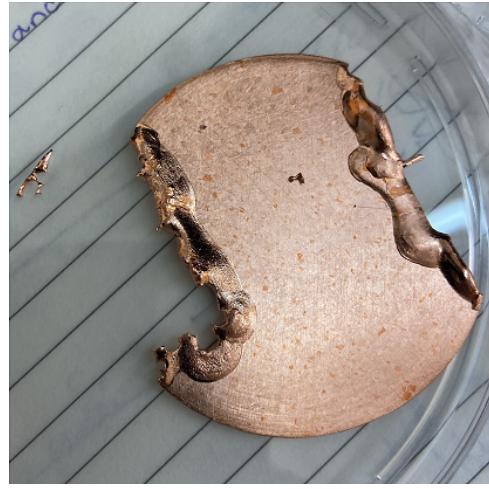
(b) Disk after being taken out from the CVD furnace. The sides that were facing the electrodes of the heater are sublimated and melted.
