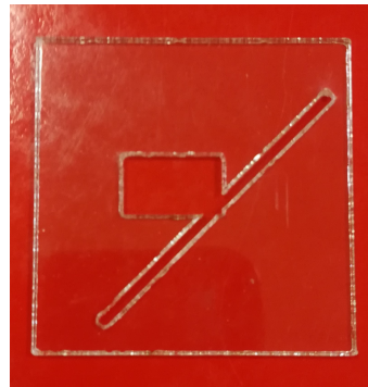
(b) Fabricated corner cutter for positioning of the insert
