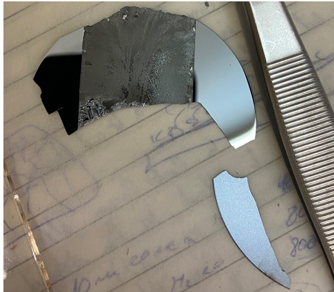
(a) Sample of Si wafer with copper foil after being taken out from the CDV machine, broken due to rapid cooling.
