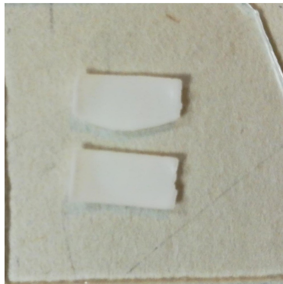
(b) Comparison between inserts that are uncut (bottom) and cut (top) with a round bottom
