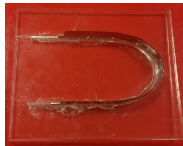
(d) Fabricated curved cutter to improve biocompatibility
