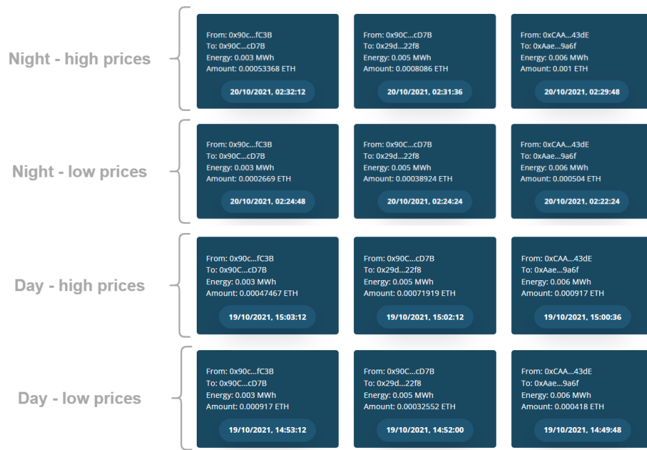
Figure 4.13: Blockchain with the results of the third smart contract, when testing all electricity price scenarios and the second situation.
