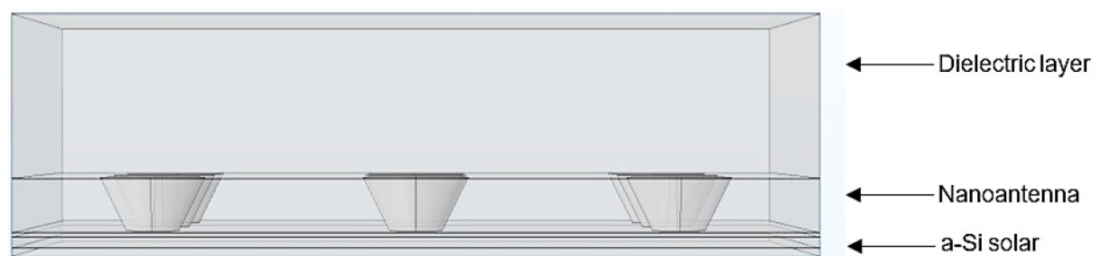
Figure 2.2: Incorporation of a nanoantenna in a a-Si solar cell. (Adapted from: [6])
