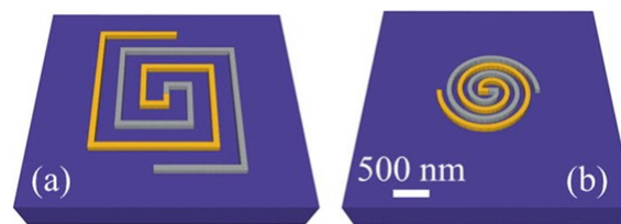
Figure 2.9: Example of Seebeck nanoantennas. (Source: [25])
