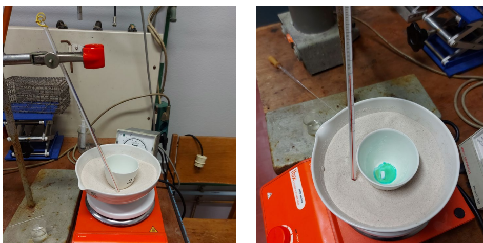
Figure 22: Incipient wetness impregnation set-up.
