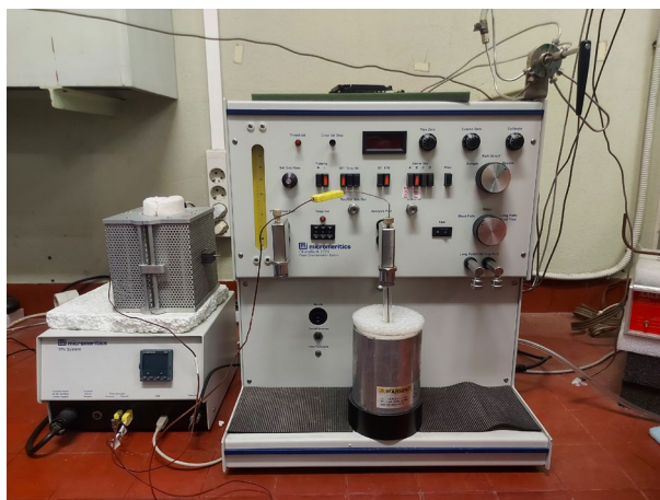
Figure 25: BET set-up in a Micrometrics ChemiSorb 2720 – ChemiSoft TPx system.
