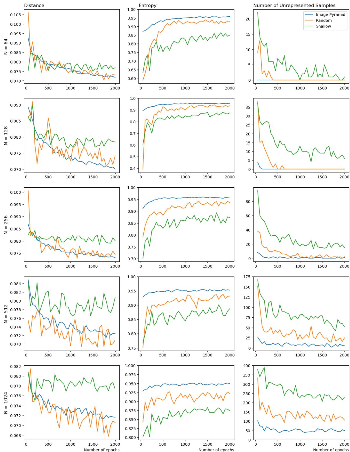
Figure 5.5: Measures for the three proposed machines regarding Mean Distance, Entropy, and Number of Unrepresented Samples on the first, second and third column respectively, with the number of train set samples N increasing on each row. The multi-level based approach showed better results on both Entropy and Number of Unrepresented Samples for all N values, while the shallow network performed worse on all measures for all experiments.
