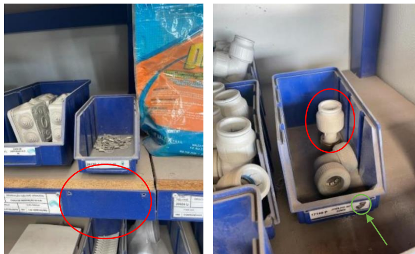
Figure 12: Lack of labeling (right) and label not respected (left)
