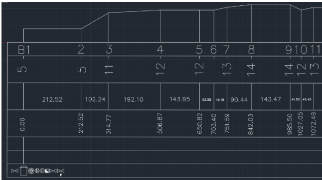
Fig. 6 – Initial section of the system, that contemplates the first pumping station (B1) and its accessories (from left to right, sectioning valve, reservoir (R1), pump, flow meter, pressure meter, retention valve, sectioning valve and bottom discharge valve)
