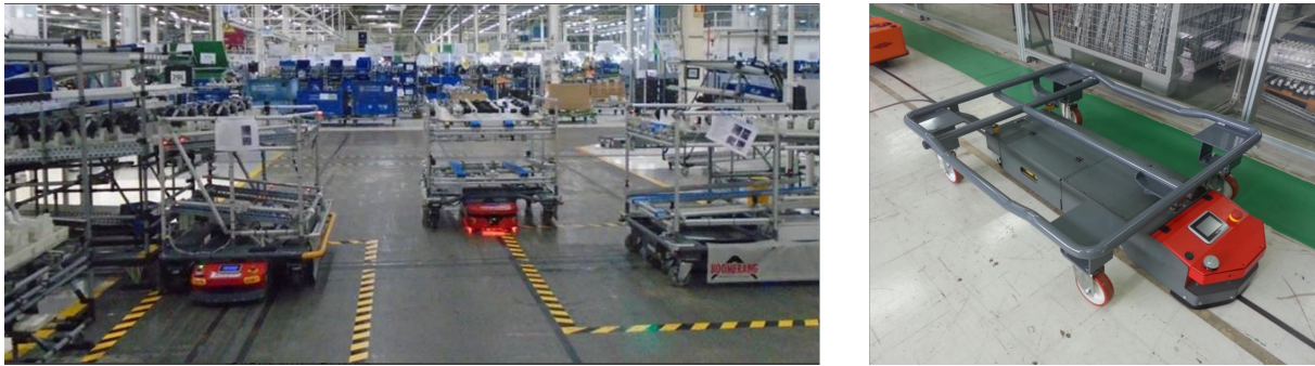
Figure 1.1: AGVs operating in the Volkswagen Autoeuropa facilities (left side). Example of an AGV transporting a rack and following a magnetic stripe of the floor (right side).
