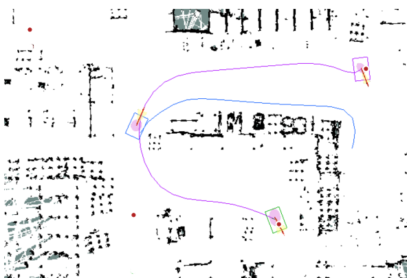
(e) t = 106.14s : R^3 begins its journey (purple curve) from the starting to the ending point of s^3 , Locations 4 and 3, respectively. R^1 is following the trajectory previously initiated (blue curve). R^2 (green) is at Location 3.
