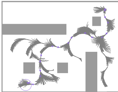
(k) Trajectory planning of R^6 . Kinodynamic RRT tree constructed (grey) and generated initial guess trajectory (purple).
