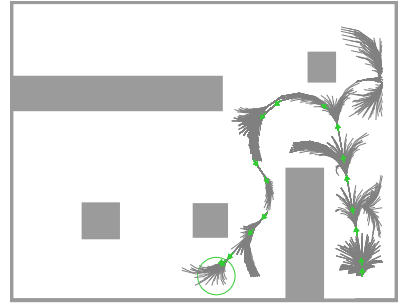
(c) Trajectory planning of R^2 . Kinodynamic RRT tree constructed (grey) and generated initial guess trajectory (light green).
