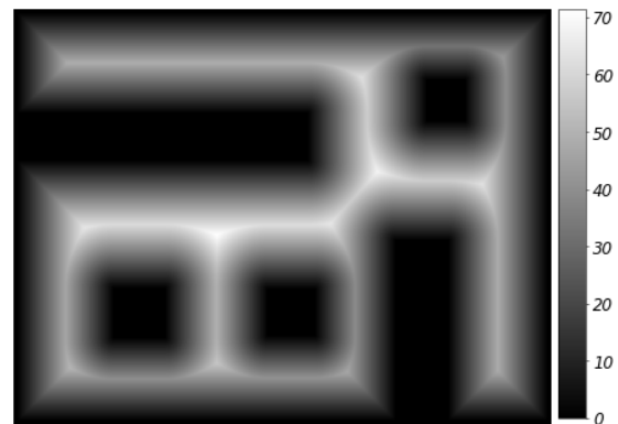
(b) Euclidean distance transform of the occupancy gridmap ( EDT_G ). Depicts the distance to the nearest obstacle.
