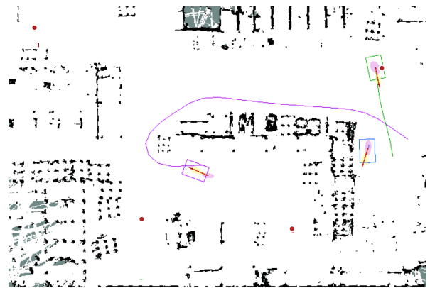
(d) t = 180.08s : R^2 finishes s^2 and begins a journey (green curve) to return to the idle zone. R^3 is following the trajectory previously initiated (purple curve). R^1 (blue) is in the idle zone.
