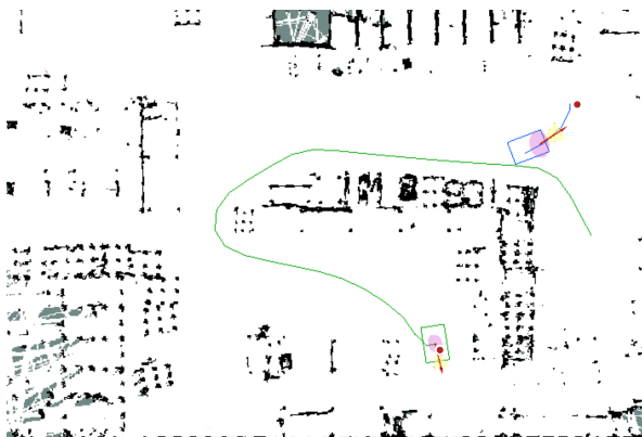
(e) t = 105.00s : R^2 finishes s^3 and begins a journey (green curve) to return to the idle zone. R^1 is following the trajectory previously initiated (blue curve).
