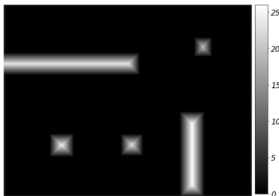
(c) Euclidean distance transform of the occupancy gridmap logical complement ( EDT_{\bar{G}} ). Depicts the distance to the nearest unoccupied area.
