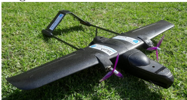
Figure 4: Developed Drag-mode System Flying Testbed.
