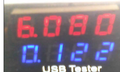
Figure C.6: Measured output voltage and current in a downwind horizontal leveled "quasi-steady" flight condition (FC6).
