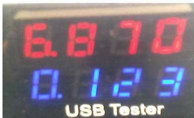
Figure C.5: Measured output voltage and current in a downwind horizontal leveled "quasi-steady" flight condition (FC5).
