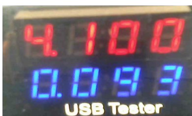
Figure C.7: Measured output voltage and current in an aerodynamic stall flight condition (FC7).
