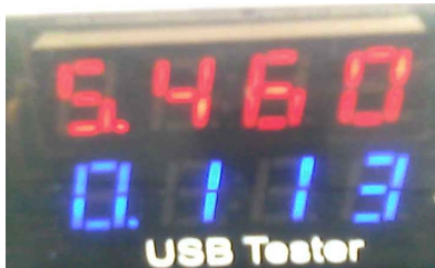
Figure C.1: Measured output voltage and current in an upwind climb flight condition (FC1).
