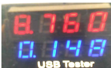
Figure C.8: Measured output voltage and current in a steep pitching flight condition (FC8).
