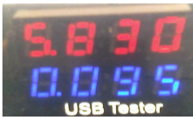
Figure C.4: Measured output voltage and current in a upwind horizontal leveled, with great turbulence, flight condition (FC4).
