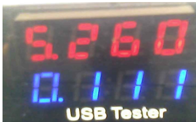
Figure C.2: Measured output voltage and current in a downwind climb flight condition (FC2).
