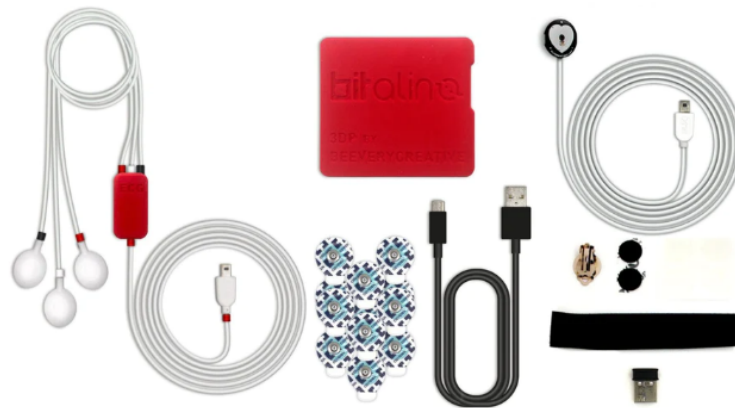
Figure 3.3: Heartbeat - Plux hardware kit capable of measuring cardiac activity measurements (e.g., heart rate and heart rate variability) by evaluating electrocardiography (ECG) and Photoplethysmography (PPG) signals.
