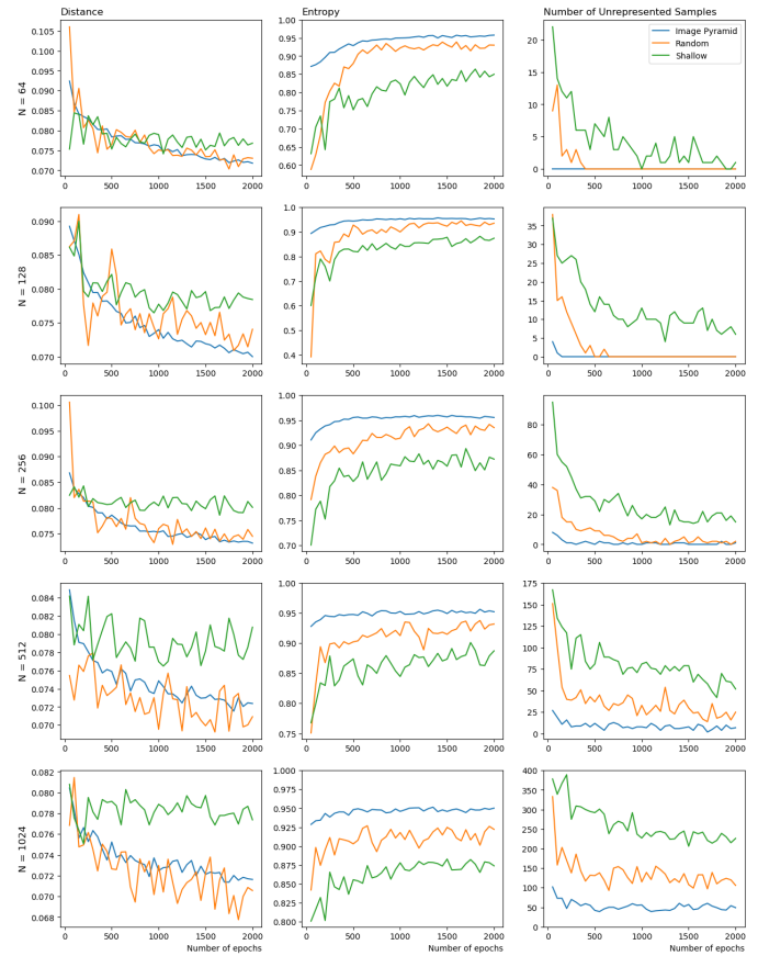
Fig. 7. Measures for the three proposed machines regarding Mean Distance, Entropy, and Number of Unrepresented Samples on the first, second and third column respectively, with the number of train set samples N increasing on each row. The multi-level based approach showed better results on both Entropy and Number of Unrepresented Samples for all N values, while the shallow network performed worse on all measures for all experiments.
