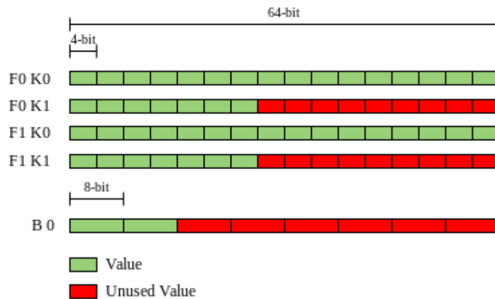
Figure 4.2: Filter and Bias data example
