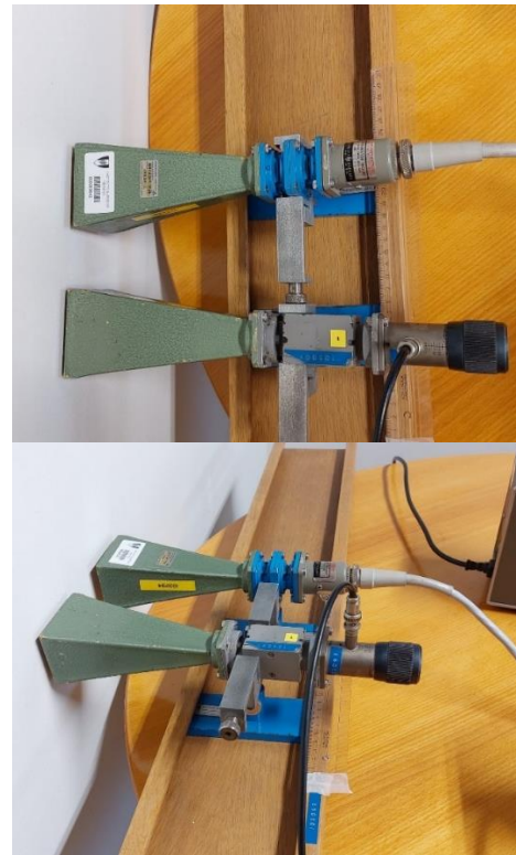
Fig. 20 - Installing the two pyramidal horn antennas in parallel with the wall
