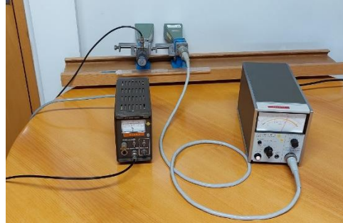
Fig. 19 - Experimental assembly of two pyramidal horn antennas with power supply and a power meter
