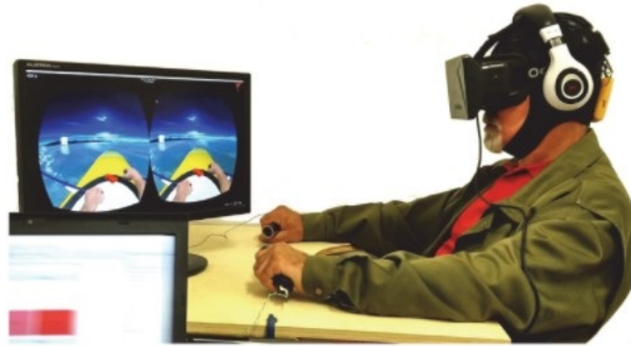
Figure 2.10: A BCI–VR experimental setup that uses the Oculus Rift VR headset, headphones, and hand controllers generating vibrotactile stimulation to interface the subject with the VR environment NeuRow [9]
