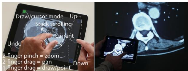
Figure 3. Touch display with interface to the left. Combination of PC screen projection and mobile device on the right. Adapted from [7].
