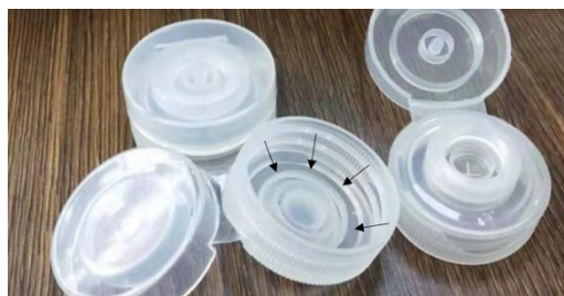
Figure 35 - PP lid indicating the positioning of the set of spikes
