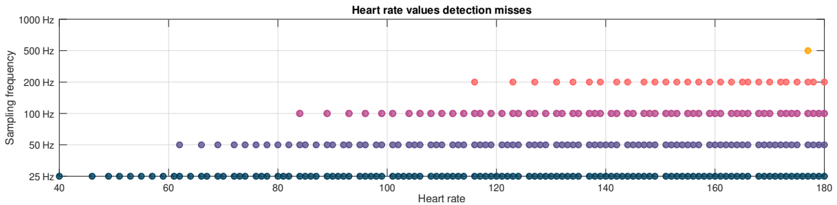
Figure 3.4: Heart rate detection misses varying with sampling frequency.
