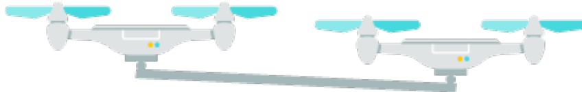
Figure 2.1: Configuration of the quadcopter bar system.
