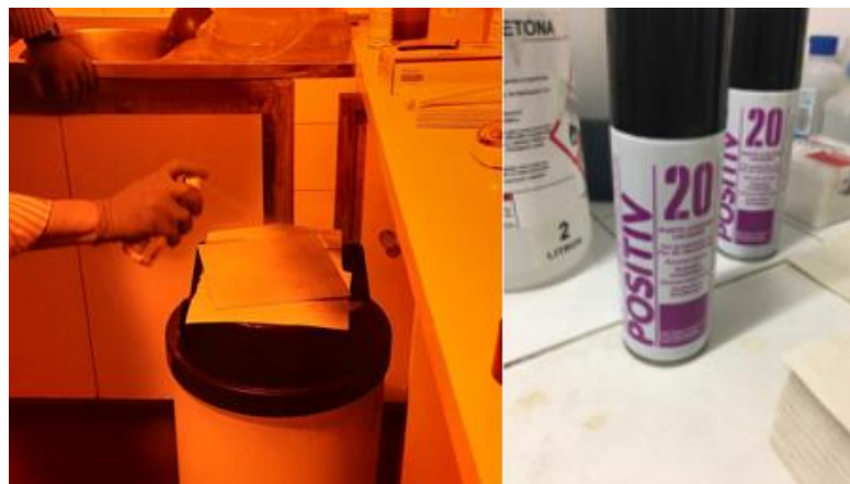
Figure 4.2 - Applying the photoresist solution Positiv 20
