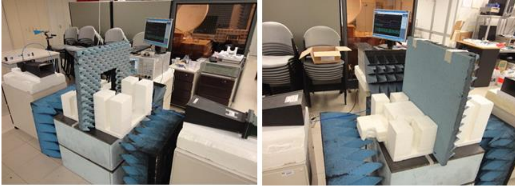
Figure 3.33 – Setup for the experimental macroscopic characterization of Eccosorb AN-75
