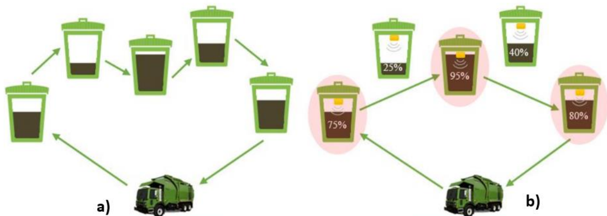
Figure 5: Waste collection routes with (b) and without (a) the ultrasonic sensor technology (adapted from Gonçalves, 2014).
