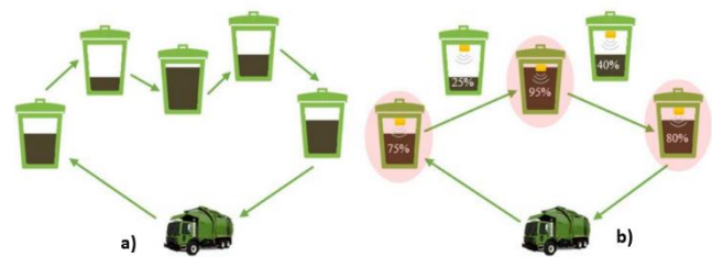
Figure 1: Waste collection routes with (b) and without (a) the ultrasonic sensor technology (adapted from Gonçalves, 2014).
