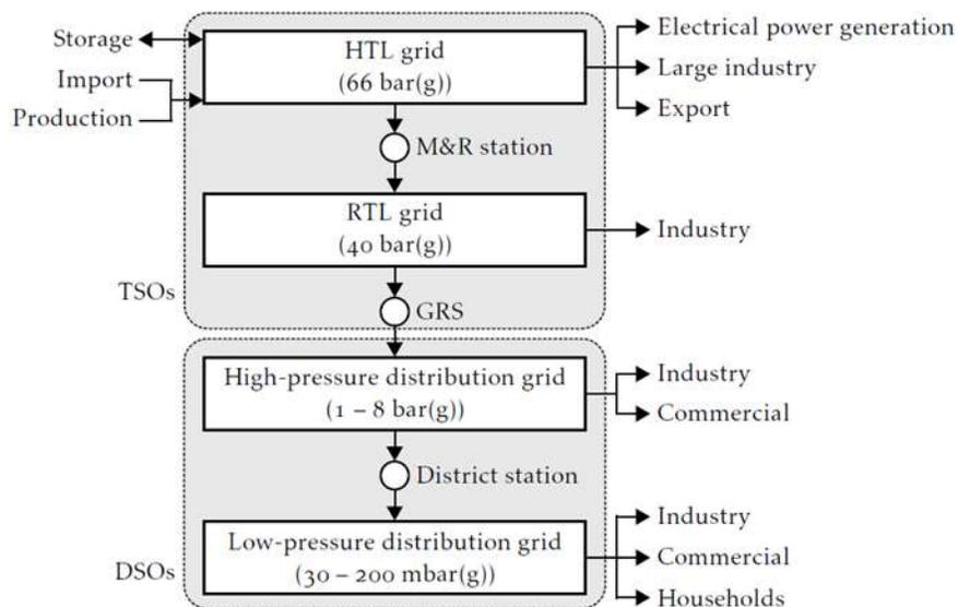
**Figure 23. Dutch gas grid supply chain [32]**
