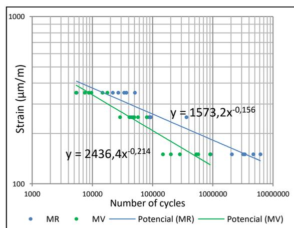
**Figure 1 – Fatigue laws obtained for MR and MV**
