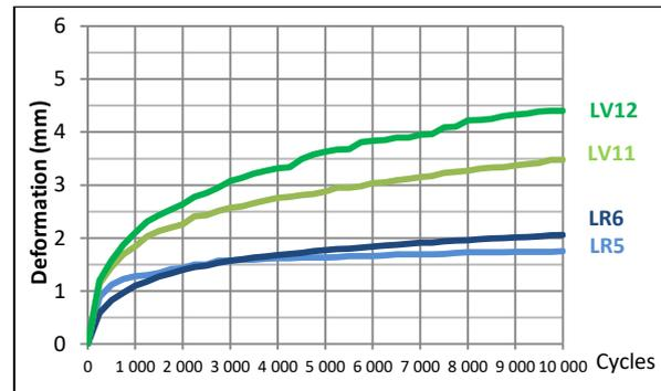
Figure 2 – Evolution of Wheel Tracking for mixtures MR (LR5 and LR6) and MV (LV11 and LV12)
