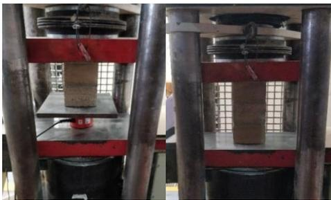
Figure 2. a) Two half blocks test b) Three half blocks test
