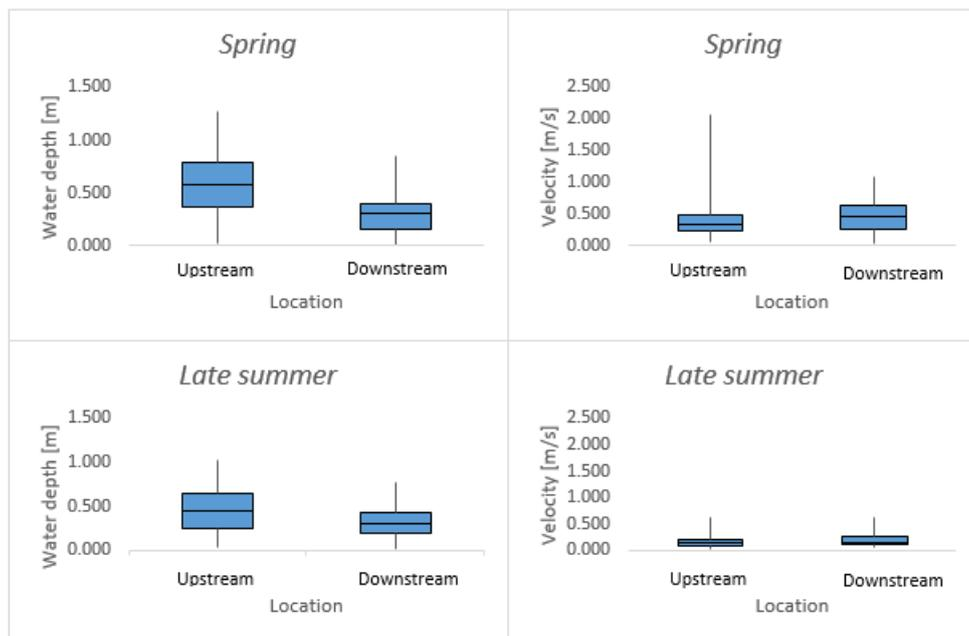
Figure 2 – Water depth and discharge velocity conditions for fishes upstream and downstream the water release from the hydropower plant, during Spring and late Summer season
