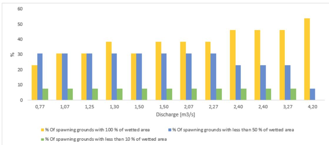
Figure 4 – Relation between spawning grounds percentage and wetted area percentage, related with each operational scenario considered for the hydropower plant.
