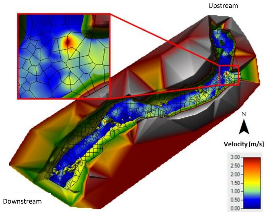
Figure 1 – Discharge velocity in the river reach considering the maximum turbined discharge ( $2,2 \text{ m}^3/\text{s}$ ) and the maximum discharge from the river natural regime ( $2,0 \text{ m}^3/\text{s}$ ).
