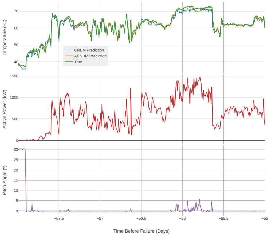
Figure 4.15: Temperature predictions for the CNBM and the ACNBM before Failure B
