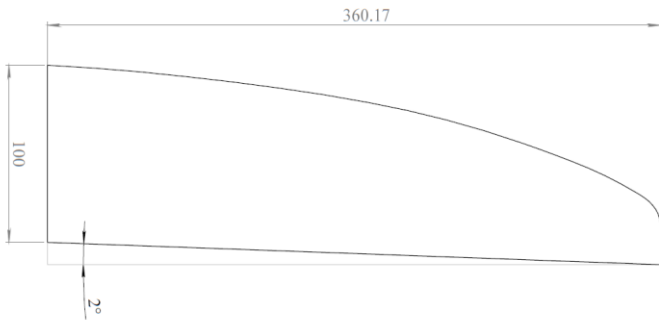
Figure 1: Slalom Windsurf board fin dimensions (all dimensions in mm and degrees)
