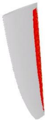
Figure 11: LSB at the Fin, Re: 5.0 \times 10^5 , 0^\circ AoA
